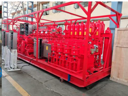
BOP control system
