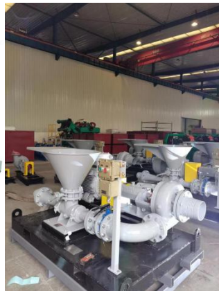
Centrifugal pump with hopeer system
